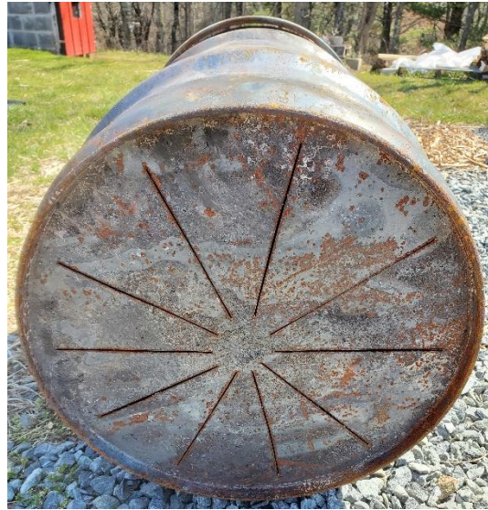
Slits cut in the bottom of the retort allow gas to escape, preventing explosion
