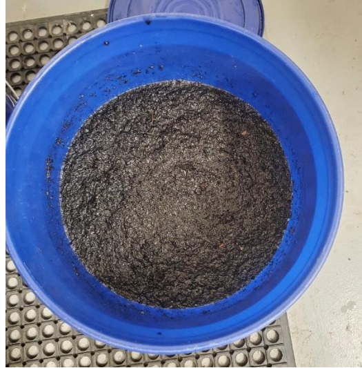
Biochar charging in anaerobic digester effluent
