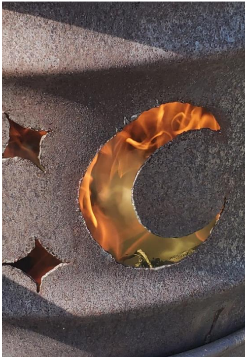
Yellow smoke within the TLUD indicates methane and other harmful gases
